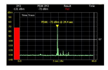
Dynamic testing identifies loose metal-to-metal connections as well as contact surface defects that might cause arcing at higher power levels. Without dynamic testing these defects could go unnoticed until activated by wind loading, tower vibration or stresses caused by temperature changes.
